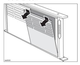
■ At the upper edge, push the grease filter down until you can pull it forward, then up and out.
